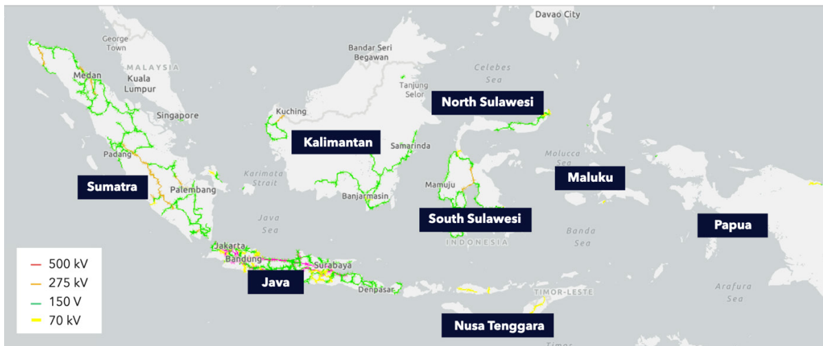
Figure 3. Power grid system, Indonesia
