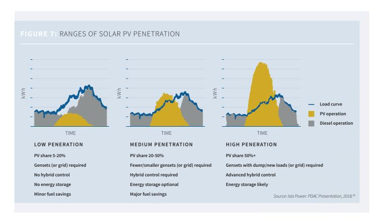
In places where there are complementary generation profiles between wind and solar sources, higher renewable penetration rates can be achieved (see Figure 8 and Box 5). When merged with storage, penetration rates can be increased further (see Box 14).
